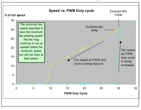
Figure 5 Type C, Operation below Minimum RPM, Min, RPM = Starting RPM
