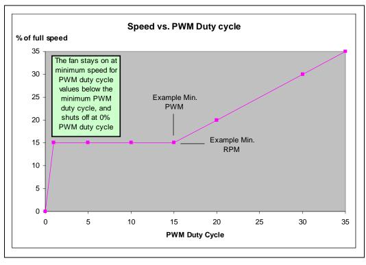
Figure 4 Type B Operation, Stay On at Minimum RPM, Off at 0% RPM
